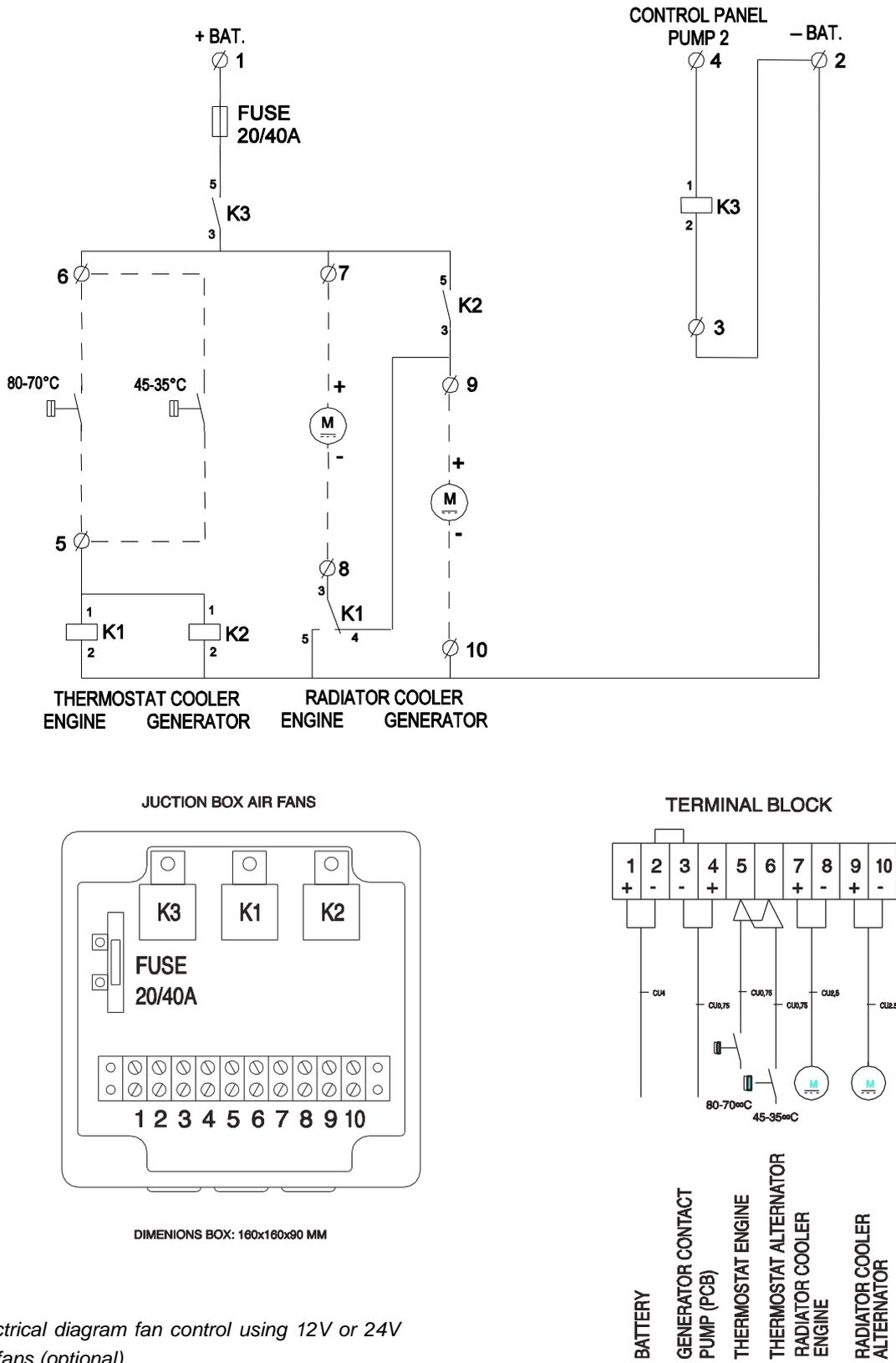
Fig. 16: Electrical diagram fan control using 12V or 24V DC radiator fans (optional)
