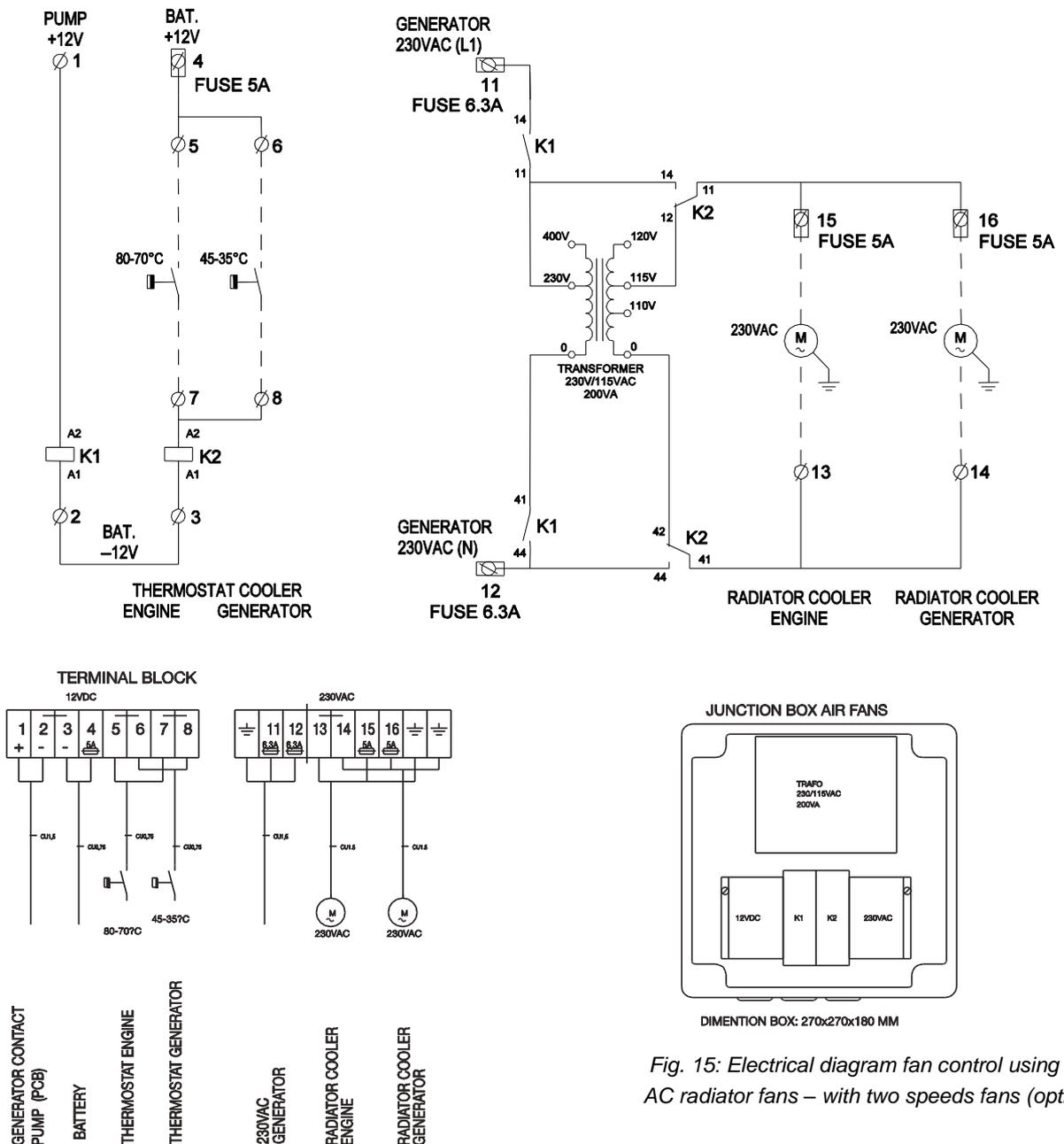
Fig. 15: Electrical diagram fan control using 230V AC radiator fans – with two speeds fans (optional)
