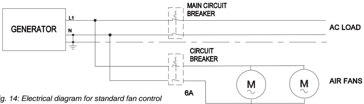
Fig. 14: Electrical diagram for standard fan control using 230V AC radiator fans
