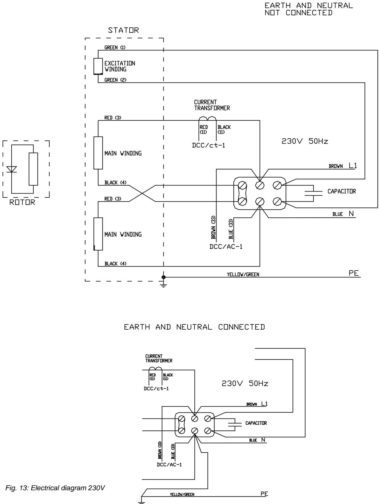
Fig. 13: Electrical diagram 230V
