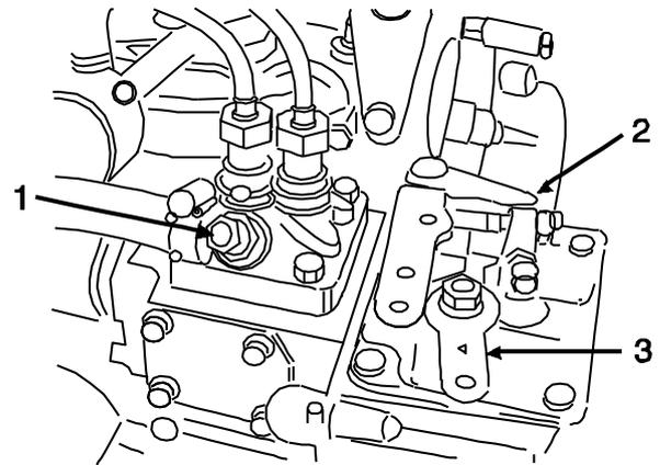
Fig. 19: Bleeding fuel lines 1 = Fuel bleeding screw
