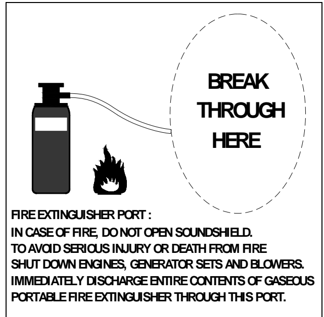
Fig. 2: Fire extinguisher port.
