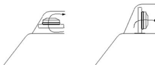
Figure 12: Two examples of top mount radiators
